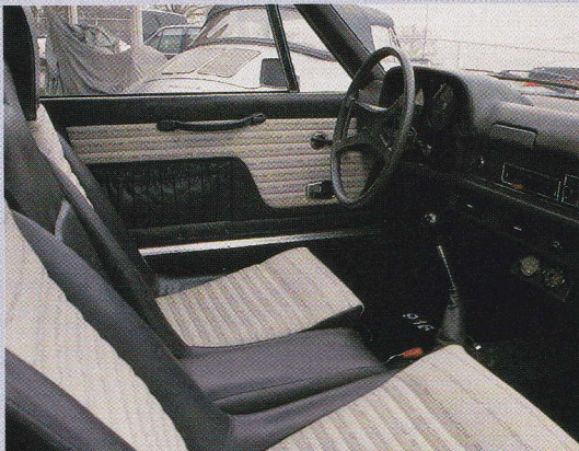
After removing the center storage console to accommodate the air conditioner, Brumos installed this two-gauge VDO instrument panel
