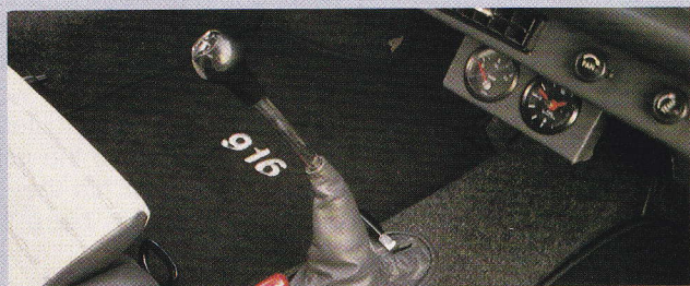
After removing the center storage console to accommodate the air conditioner, Brumos installed this two-gauge VDO instrument panel
